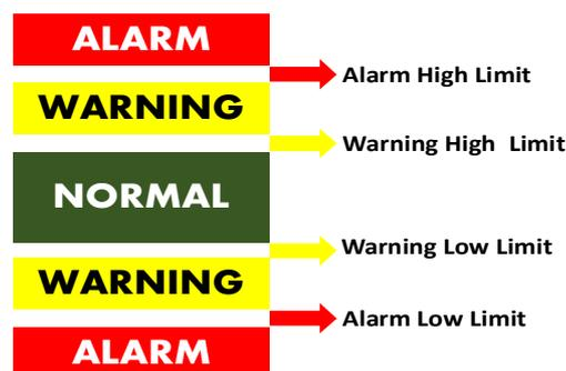
Four treshold values are assigned to the sensor which Sensplorer alerts when exceeded up or down.
