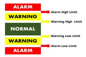
It continuously measures the RMS value of three phases and compares with the assignd limits. It activates the assigned rules in case of any limit exceed
