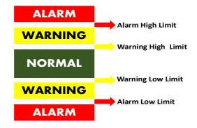
Four treshold values are assigned to the sensor which Sensplorer alerts when exceeded up or down.
