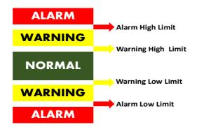
Four treshold values are assigned to the each sensor which Sensplorer alerts when exceeded up or down.
