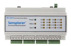
The Sensplorer 16-port Dry Contact Sensor monitors relay outputs of device and sensors in terms of their status. A dry contact output can be one of in two status: "1"(closed) or "0" (open). Devices and sensors define the one state as Normal while the other as Alarm. When they are connected to Sensplorer Dry Contact Sensor, Alarm and Normal state is assigned with respect to its documentation.
