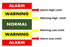
Four treshold values are assigned to the each sensor which Sensplorer alerts when exceeded up or down.
